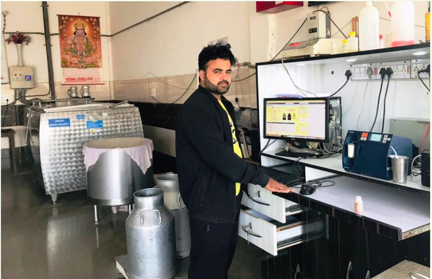
Bulk Milk Cooler and Milk Adulteration testing machine at Pandori, Garhshankar, Hoshiarpur, under NPDD
