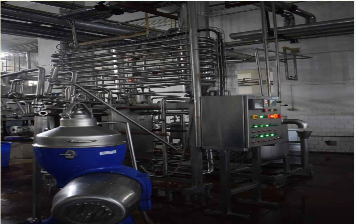
5 KL HTST pasteurizer, East Khasi Hills District under NPDD scheme
